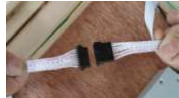
Figure B-9: Connecting the control panel plug.
