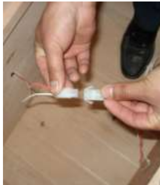
Figure B-5: Connecting the heater's plug
