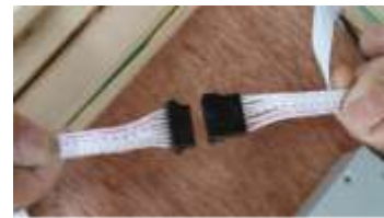
Figure C-9: Connecting the control panel plug.
