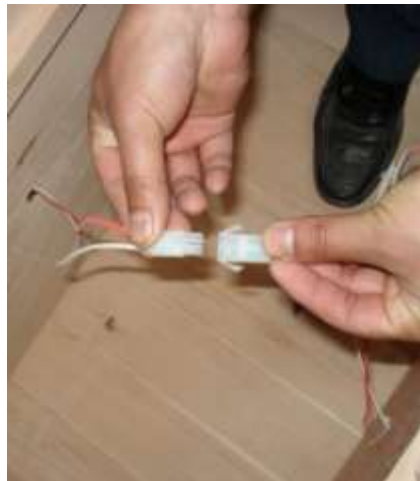
Figure A-5: Connecting the heater's plug
