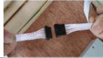
Figure A-9: Connecting the control panel plug.
